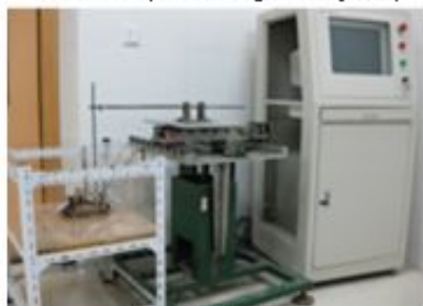
超声场测量系统 ( Measuring system for ultrasound field )
